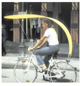
In order to ensure an absolutely unchanged riding quality, **utmost priority** has been attributed to free **visibility and optimum freedom of movement** when designing the protective device. It is an important factor that the roof covering does not deform during cornering.
